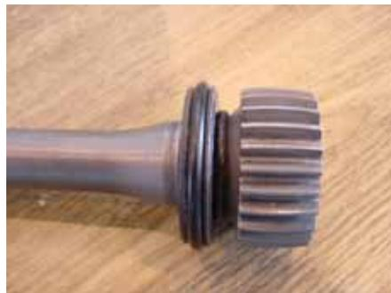
*New shaft with seal & spacer*
