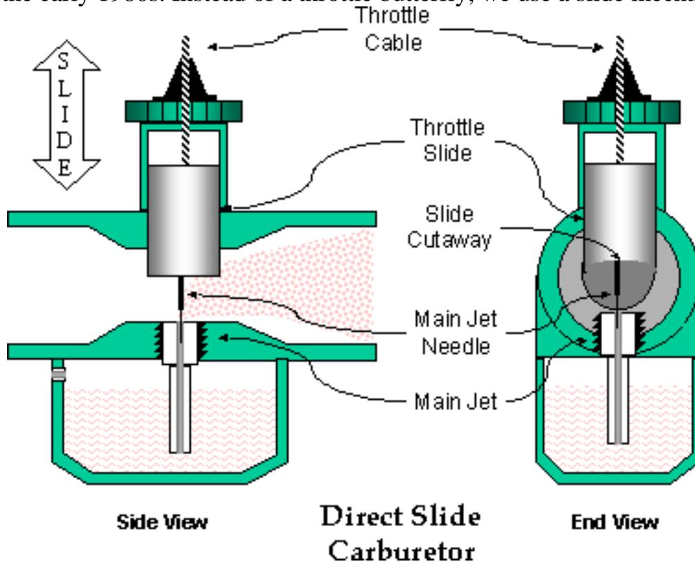
off the supply of air to the engine. But now, because we are varying the size of the venturi, we have to also vary the size of the fuel jet. No problem, as we'll just add a tapered needle to the bottom of our slide that runs down into the jet at partial throttle openings. Once we open the slide all the way, we are back to a standard venturi size, the needle is pulled out of the jet and we're back to our fixed air to fuel ratio. At least we are if the jet is the
